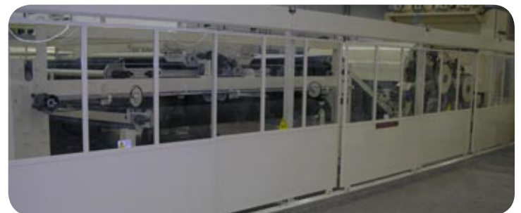
Sliding panels with wide inspection windows and sensor-type locking devices, in compliance with the European regulations.
