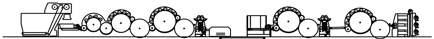
● 4 carding groups + Breast roller with 1 broad band feed ● 4 carde + avantreno con 1 traversatore ● 4 cardas + avandrén con 1 transportador cruzador
