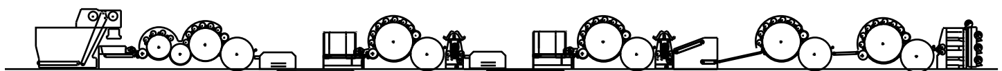
● 5 carding groups + Breast roller with 2 broad band feed + 1 parallel lapper, mod. AFP50 ● 5 carde + avantreno con 2 traversatori + 1 faldatore parallelo mod. AFP50 ● 5 cardas + avandrén con 2 transportadores cruzadores + 1 plegador paralelo mod. AFP50
