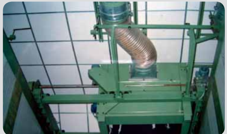
Bin feed system by movable mouthpieces or stationary/rotating mouthpieces or by a moving-displacing feed condenser, as shown in the picture
